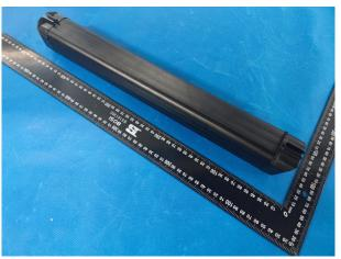
**こ**□□□□ Rechargeable Li-ion Battery Model:CZM240701 Voltage:36V Capacity:10Ah(360Wh)
